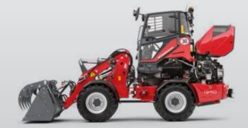
Good service accessibility. The driver's cab or cabin can be tipped to the side. This allows uncomplicated access to the engine, hydraulic system and electrics. This greatly simplifies the monitoring and maintenance of the machine. The arrangement of components in the inner machine has been further optimized.
