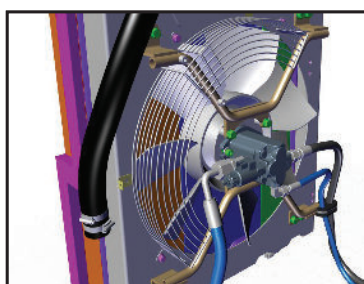
Hydraulic Fan Drive for Radiator
